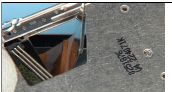
38. Shift the slider into position shown to reach the maximum recess. Slot the connector through the slider.
